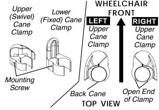
FIGURE 1 - INSTALLING/REMOVING CANE CLAMPS
